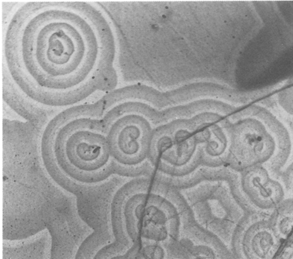
Figure 8 A group of interacting dislocation spirals and loops ( \times 150 ).
