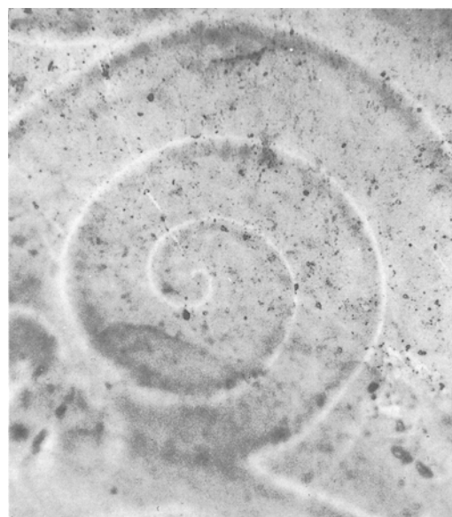
Figure 2 A circular spiral originating from a single dislocation ( \times 470 ).
