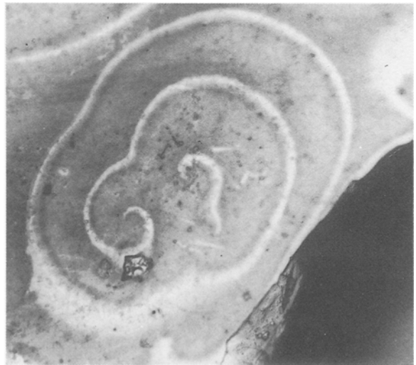
Figure 11 An expanding spiral spreading from multiple sources ( \times 500 ).
